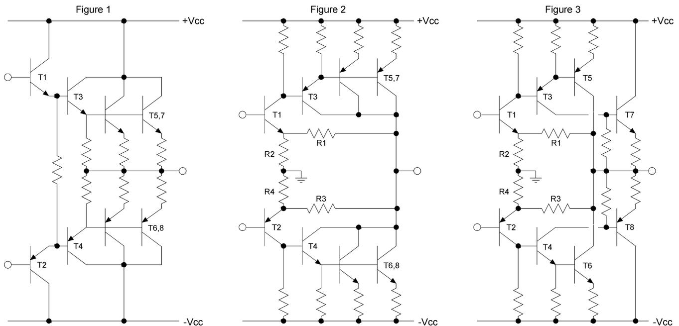
**Figure 1** is a classic triple Darlington stage where each successive transistor is driven from the emitter of the previous stage. This arrangement features a current gain of approximately 10 and a voltage gain of 1. It is reasonable linear but has a few limitations:
